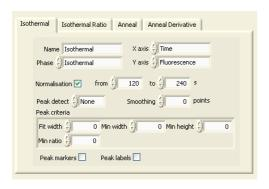
Normalisation allows all the fluorescent signals to be normalised/back grounded over a defined period of time.
