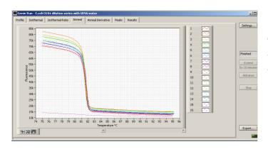
The 'Anneal' tab plots the fluorescence of each well versus temperature in an annealing curve.
