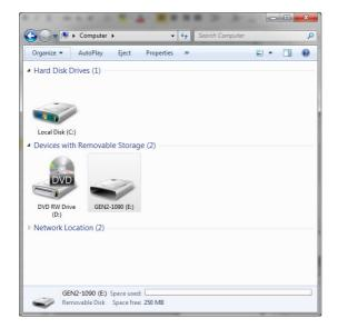
Genie® II is now visible as a USB drive in 'My Computer' and the name appears as the instrument's serial number.
