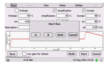
A prompt will ask whether the experiment is to be run on block A, block B, or both. Only the block or blocks that are available (i.e. not already running) will be offered.
