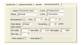
Simple: The software looks at the peak and assigns the peak to the highest plotted point. Multiple peaks can be detected.
