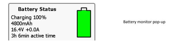
*IMPORTANT!* Genie® II's internal battery will only charge when the instrument is plugged into mains electricity and the instrument is switched on. Genie® II can then be shut down using the 'Turn Off' button within the 'Utilities' menu. The LED above the display will glow brightly until the battery is fully charged. At this point Genie® II can be switched off using the switch on the rear.
