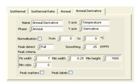
Full: The software curve fits and assigns the centre of a peak and can report multiple peaks. It also performs sub-point interpolation.
