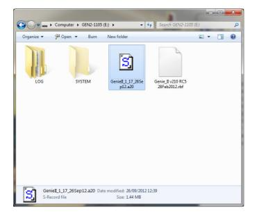
To install the updates, connect Genie® II to a computer. Navigate to 'My Computer' and open the Genie® II drive. The drive is named after the instruments serial number, e.g. GEN2-1105. Copy and paste (or drag) the firmware or FPGA software files onto Genie® II.
