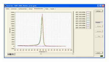
The 'Anneal Derivative' tab shows the derivative fluorescence of each well plotted against temperature, thereby giving the data as a peak.
