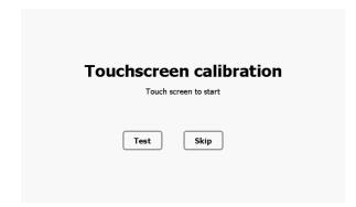
Touching anywhere on the screen with the exception of Test or Skip will invoke the touchscreen calibration
